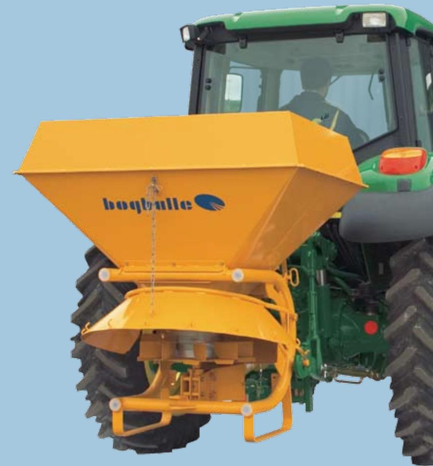
**Stepless working width** from 1-8 metres - depending on spreader type.
