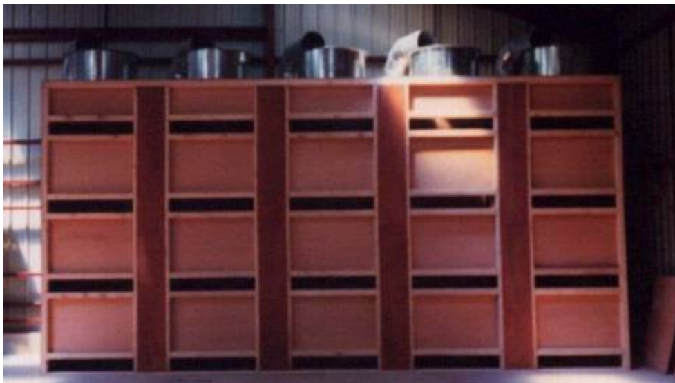
Example of 5 ventilation towers for 4 boxes high.
