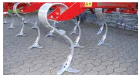
Vibro Flex Mixing kapa (VFM).
