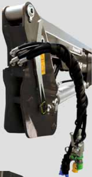
Original hydraulic hose connection system in loader connection clamps stops unwanted hose movement near exhaust and front window.
