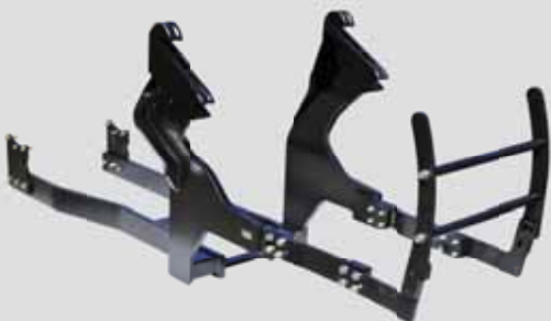
The subframe construction is unique with its stiffness and solidity. It also assures easy access to all service points of the tractor.
