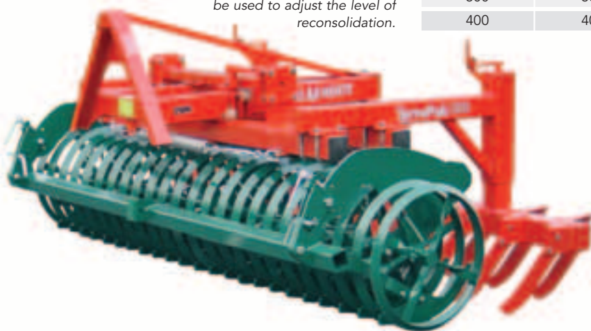
The front harrow blades have adjustable working angles – overload protection as standard.
