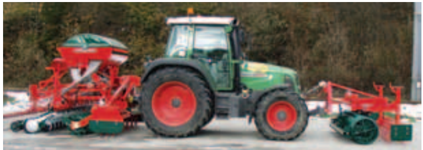
Multi-functional: Soil preparation with the VN Terrapak front roller with simultaneous sowing with the VN MasterDrill A.
